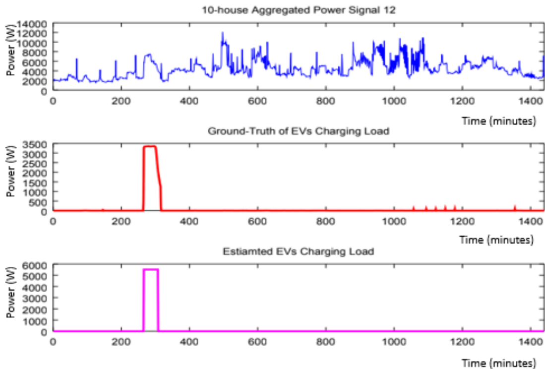
Figure 33. One day of EV consumption disaggregation
