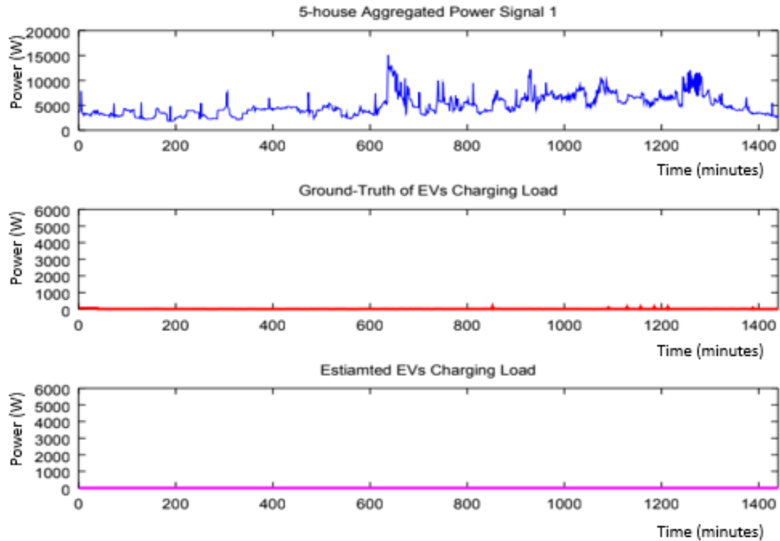
Figure 34. One day of EV consumption satisfactory disaggregation
